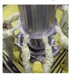
NASA is partnering with Y-12 and others on a reliable, efficient, kilowatt-size fission power system for future space missions. The prototype system is fueled with highly enriched uranium alloy components produced at Y-12.
